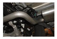
5. Install the Passenger side muffler assembly onto the factory pipe and into the factory rubber grommets. Do not tighten.
