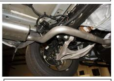
4. Install the driver side muffler assembly onto the factory pipe and into the factory rubber grommets. Do not tighten.
